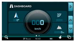
Route  $\Rightarrow$  Trip page  $\Rightarrow$  Left tab  $\Rightarrow$  Dashboard page The Dashboard has no tappable buttons, but it tells you a lot of useful information. It features a speedometer, compass, altimeter, a precision GPS signal strength indicator and your current GPS coordinates.
