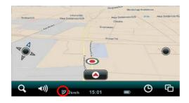
This displays your GPS signal strength. Three yellow bars indicate the maximum GPS signal strength (within a 5 meter accuracy). Fewer yellow bars indicate a progressively weaker, less accurate, GPS signal. Three red bars indicate the absence of a GPS signal.
