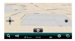
Located along the top and bottom of your screen (together with the Status Bar) in Map View in portrait mode and just along the bottom in landscape mode, the Control Bar features the Search button, the Driving Options button, the Last Page Accessed field and the Main Menu button.
